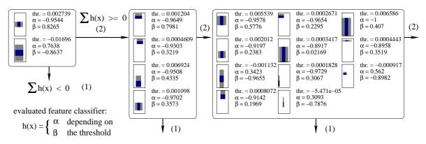
Figure 3: The first three stages of a cascade of classifiers to detect an office chair in depth data. Every stage contains several simple classifiers that use Haar-like features.
