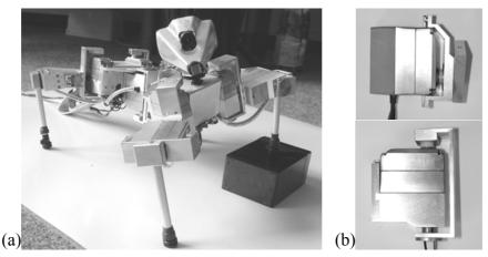
Fig.5 The first prototype of the Robo-Salamander robot (a), constructed with the joint-modules of the AIS-Walking-Robot-Kit (b)
