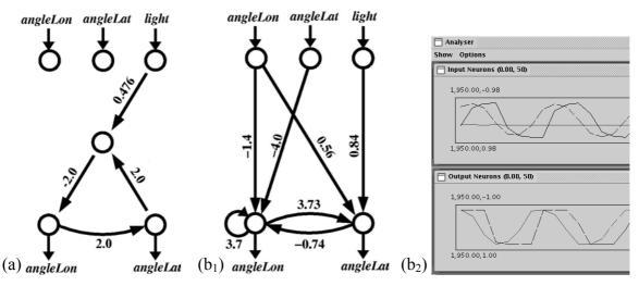
Fig.7 Evolved networks for the centre motors of the salamander (phototropic task): a simple oscillator module (a) with the proper phase shift to move forward and a more advanced one (b<sub>1</sub>) with a smoother, more adaptive walking pattern (b<sub>2</sub>).
