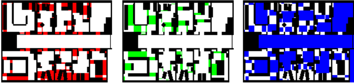
Figure 3: An environment segmentation based on the main axis clearance map with (a) narrow passages, (b) passages, and (c) free passages.
